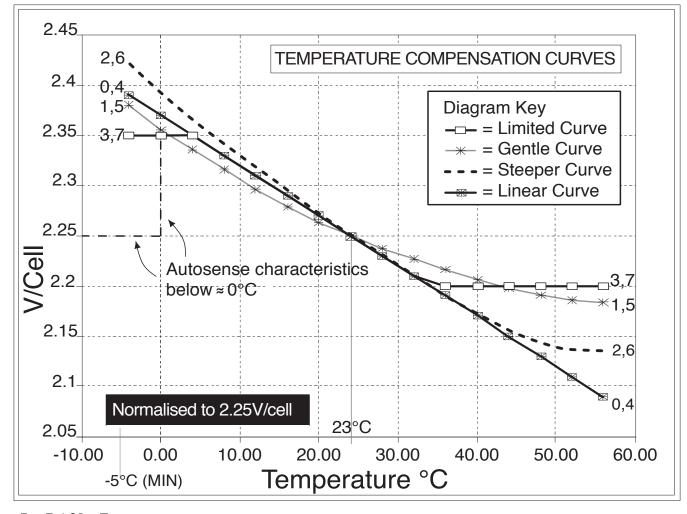
Fig. 7.4.3B - Temperature compensation curves
