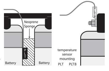
Fig. 7.4.3A - Attaching a Temperature Sensor to a battery
