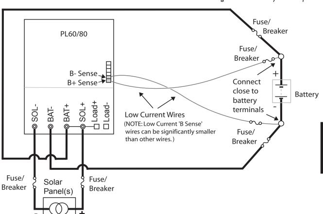
Fig. 7.5.4A - Second Battery Control
