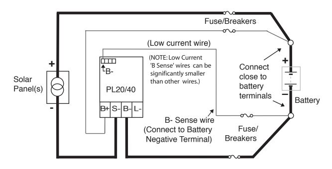
Fig. 7.5.3A - Battery Sense Input
