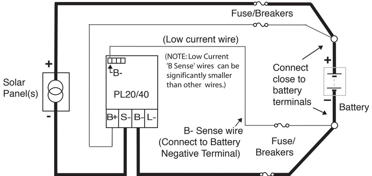
Fig. 7.5.3A - Battery Sense Input
