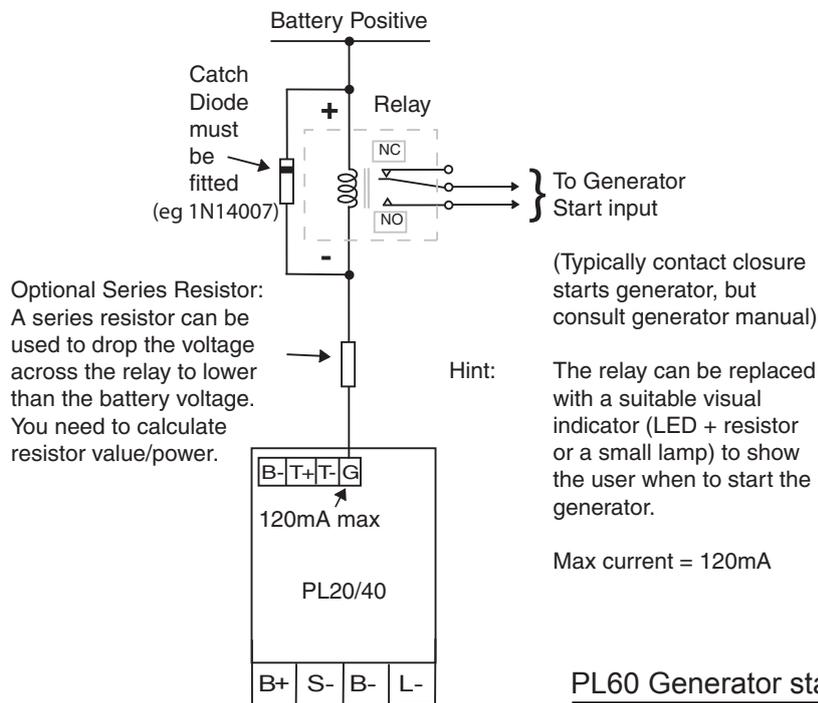
Fig. 2B - PL20/40 Generator start relay wiring
