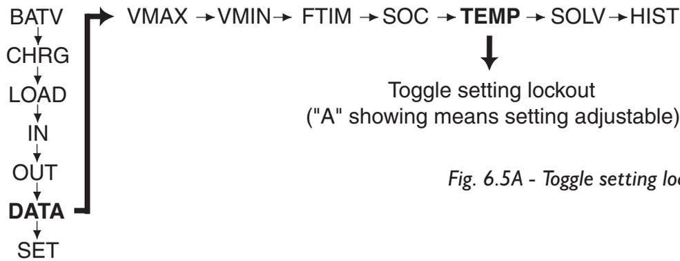
Fig. 6.5A - Toggle setting lockout
