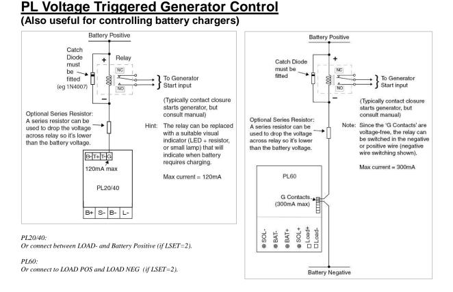
Typically, generators require a contact closure to start. The generator's start input usually requires a low current external contact closure to turn on. Please consult your generator manual for details. NOTE: The PL regulator does not manage the start-up sequence of the generator. It provides an output that stays active for the duration the regulator wants to run the generator.
