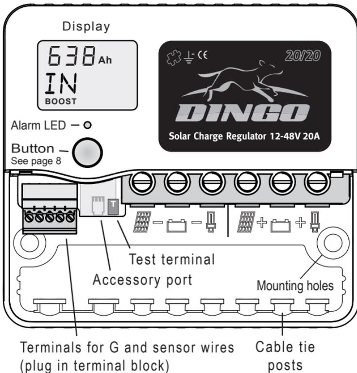
Screw wires into the high current terminals ***tightly*** in the order listed on page 6.
