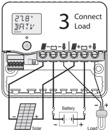
c. Test the solar panel connection by touching the positive (+) wire from the solar panel onto the Test terminal (T).
