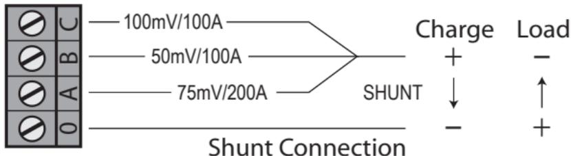
The shunt should be arranged so that the end connected to the “0” terminal is more positive for load information and more negative for charge information. If you get this wrong, there will be no damage, simply swap the wires to the shunt.
