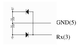
The Dingo uses an isolated "port powered" RS-232 connection, meaning that the circuitry uses a small amount of power from the device that it is connected to.
